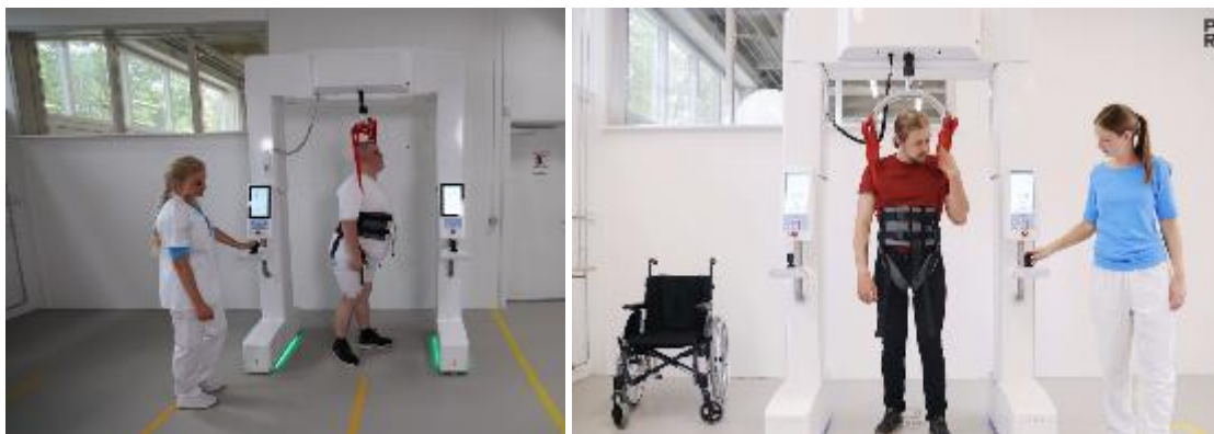
Figure 3 Current manual process gait training with PTR robot
