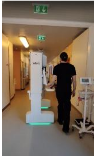
Figure 13 Operator driving robot via joystick to destination
