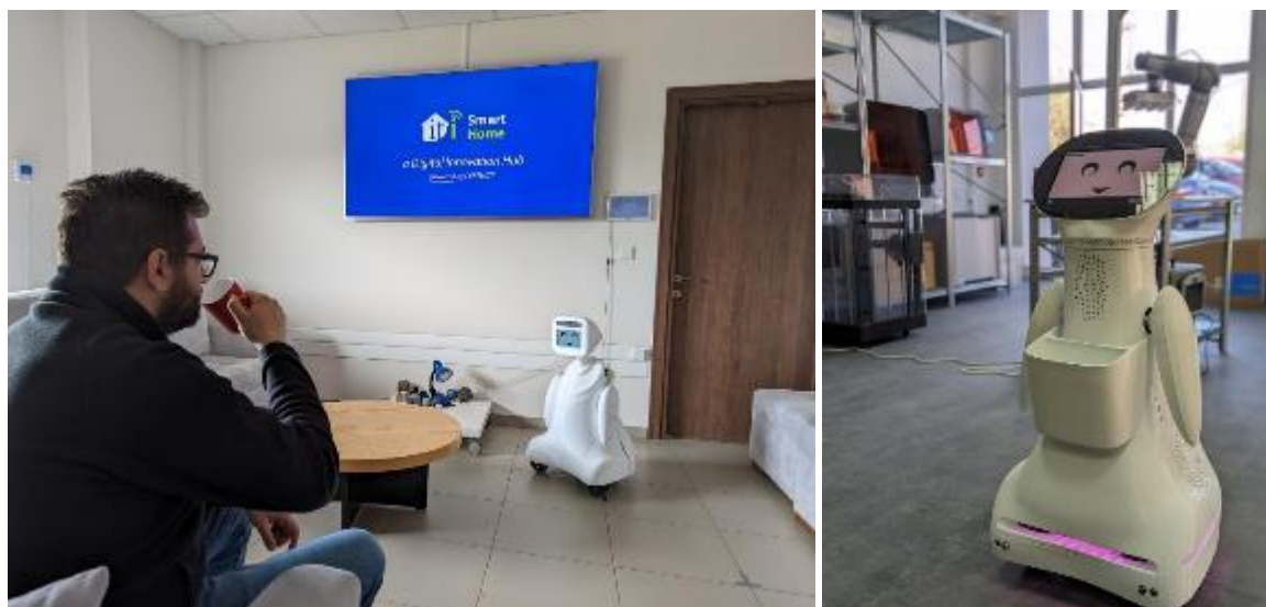
Figure 4 Current robots from CERTH performing human action recognition & receptionist tasks
